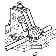
**!** To allow safe drainage of the content of the boiler if there is a risk of frost, an automatic aeration valve must be fitted to the warm water supply of the boiler. Standard for all warm water devices from Truma.
