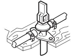
For the Trumatic C heating system, the FrostControl replaces the electrically operated safety/drain valve ELASI.
